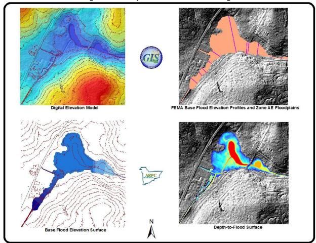
Figure III.2: Depth-to-Flood Workflow Diagram
