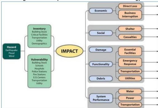
Figure III.1: Conceptual Model of HAZUS-MH Methodology
