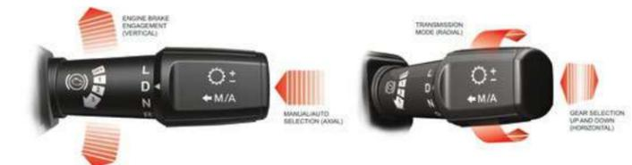
▶ The innovative stalk shifter is mounted on the steering column, allowing you to easily reach and smoothly operate shifting and engine braking while keeping your eyes on the road and your hands on the wheel.
