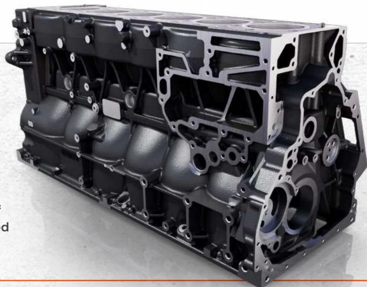
The **crankcase** is constructed with North America’s first big bore Compacted Graphite Iron (CGI) design for 75% higher tensile strength and 45% greater stiffness while reducing weight, noise and vibration.
