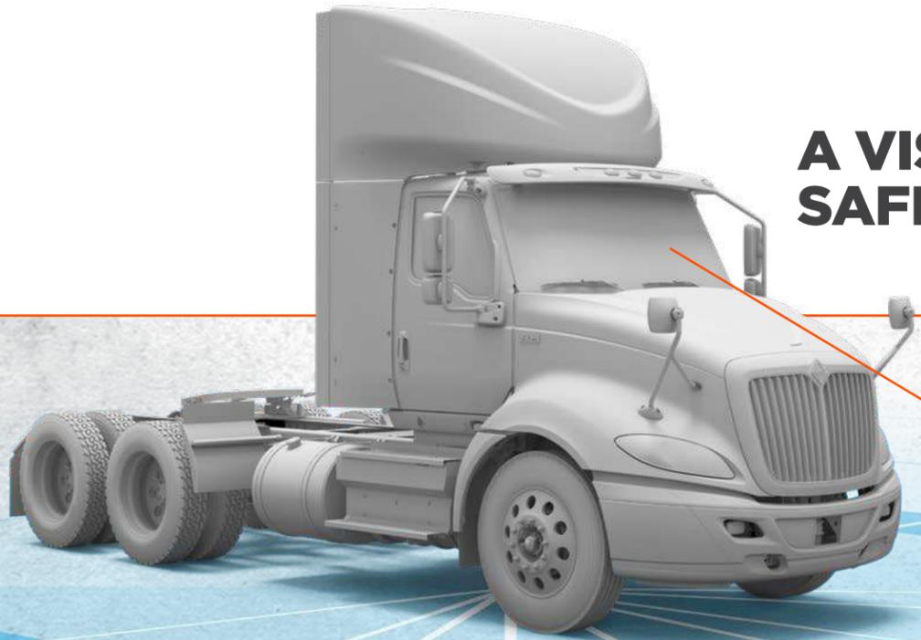
Forward visibility is among the industry's best at as little as 21'. This means objects closer to the vehicle are more visible to the driver, improving safety.
